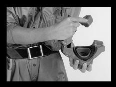
Remove one nut completely, while the other nut should be loosened enough to enable the Quik-T™ to be openen sufficiently wide to slip over pipe.
