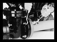
Make sure te mating flange face is free of any indentation which may prevent a good sealing. Align the Quikflange<sup>TM</sup> bolt throughout the hole of the mating flange. Handtighten the nut. Insert the next bolt opposite to the first, and add the remaining bolts in the same way. Make sure the gasket is properly positioned between the flanges. Thighten all nuts evenly with a minimum of 200Nm torque.
