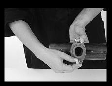
■ Place the QuikletTM over the hole on the pipe axially aligned with the hole. Make sure the leading edge of the gasket does not intersect with the hole and sits smoothly over the pipe's surface. the throat properly placed inside the hole. Check this by gently moving the Quiklet™, pushing it down at the same time.
